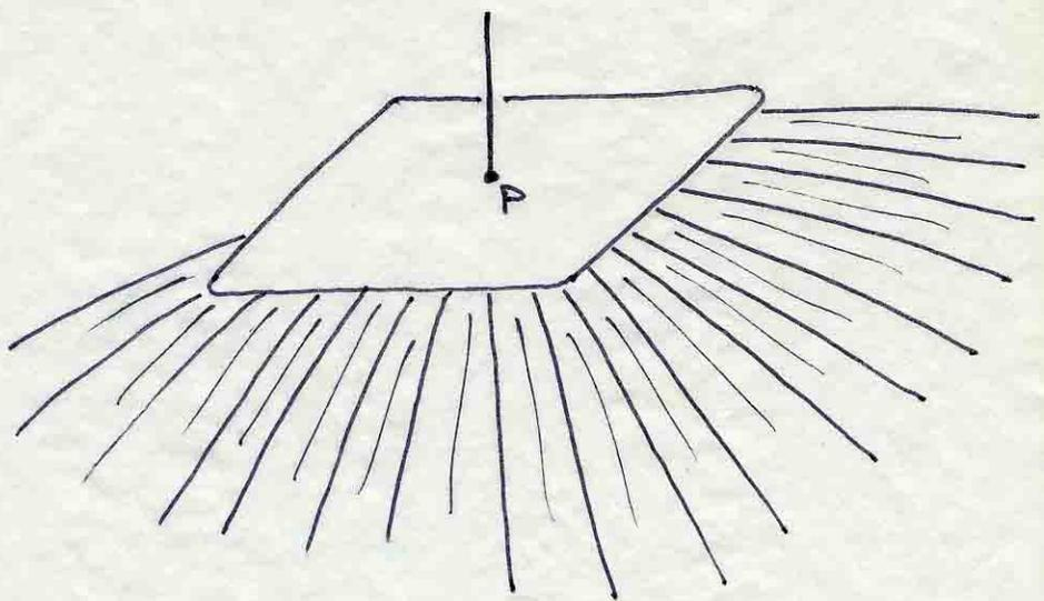
A light ray that hits a curved mirror will reflect in the same direction as if it were hitting the touching plane at the point of impact
